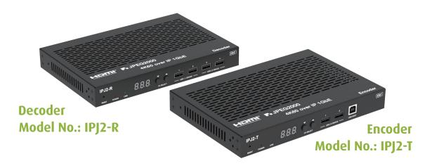
MTC IPJ2 AV over IP Series provides one of the most advanced 1G IP Streaming solutions on the market. It allows easy extension and supports up to 4K60 4:4:4 over 1GB network. This low-latency and versatile solution consists of individual transmitter and receiver units that can be configured in various combinations. The system is based on Linux for software development, which provides flexible control methods.
