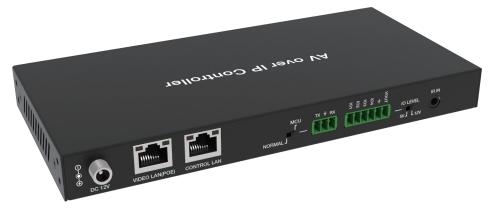
MTC IPCTL Video over IP Controller is used to control and manage JPEG2000 IP products. It supports dual 100M network ports, which can realize dual-network isolation of the control network and multicast video distribution network. Built-in WebGUI, TCP and RS-232 control are supported.
